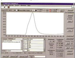
The SI400 Spectroradiometry software provides capture and display of spectra to analyze lamps, LEDs, luminescent materials and displays (below). Absolute radiometry is performed using a calibrated light source as reference. Relative radiometry can be performed using any arbitrary reference.
